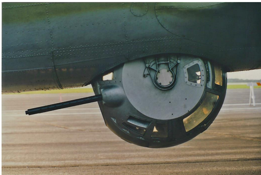
Ball turret gun position on the underside of the plane B-17G "Nine-O-Nine" (Jeff Rand, 1992 June 30)
