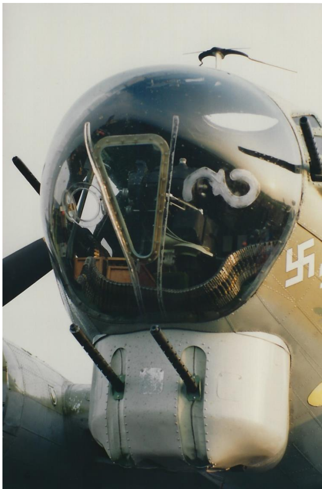
Bombardier station and chin turret, plus two cheek guns B-17G "Nine-O-Nine" (Jeff Rand, 1992 June 30)
